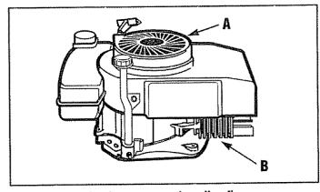
Figure 29: Air intake screen and cooling fins.
